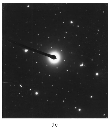
Figure 10 (a) TEM micrograph of a spherical silicon nitride grain attached to a larger silicon nitride grain; (b) SAED with diffraction spots from both grains.
